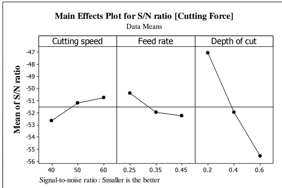
Figure 3 Main effect plot for cutting force
