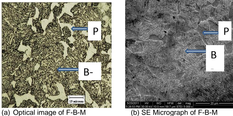
Figure 1(a) Optical and (b) Scanning electron micrograph showing polygonal ferrite and bainite-martensite colonies in the multiphase microstructure. (Sivaraman et al. 2015)
