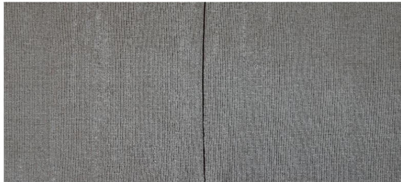
Figure 3.1 Sample RGB image (defect type : missed yarn)
