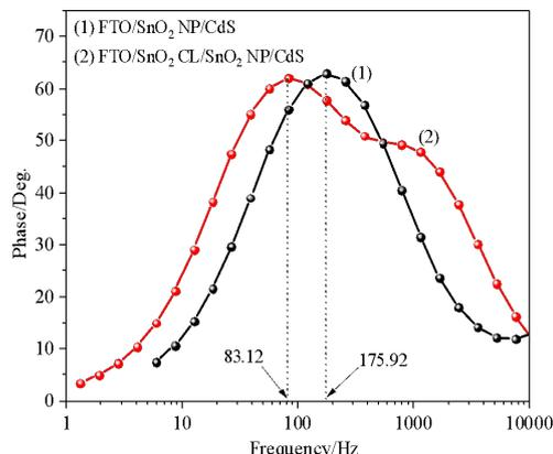
**Figure 4:** Bode phase plots of CdS QDSSCs (1) without and (2) with the SnO<sub>2</sub> compact layer in the photoanode, under the illumination of 100 mW cm<sup>-2</sup> with AM 1.5 spectral filter.
