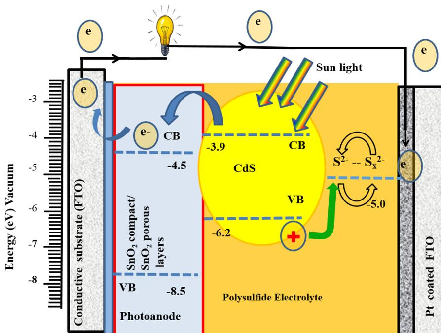
**Figure 5:** Energy band diagram of SnO<sub>2</sub> and working mechanism of CdS sensitized SnO<sub>2</sub> photoanode with compact SnO<sub>2</sub> layer.
