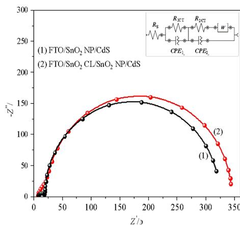
**Figure 3:** Nyquist plots of CdS QDSSCs (1) without and (2) with the  $\text{SnO}_2$  compact layer in the photoanode, under the illumination of  $100 \text{ mW cm}^{-2}$  with AM 1.5 spectral filter.
