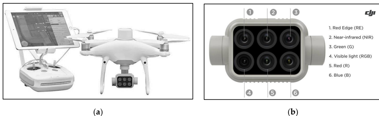
Figure 4. UAV and camera used in this study: (a) DJI P4 with remote controller and (b) RGB sensor for visible light imaging and five monochrome sensors (Source [54]).
