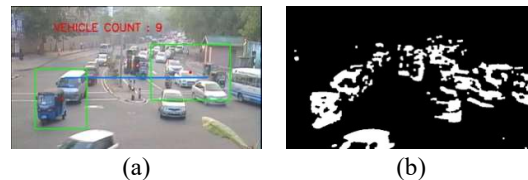
Figure 03: (a) Sample frame for detection and counting vehicle (b) Grayscale image of the sample frame
