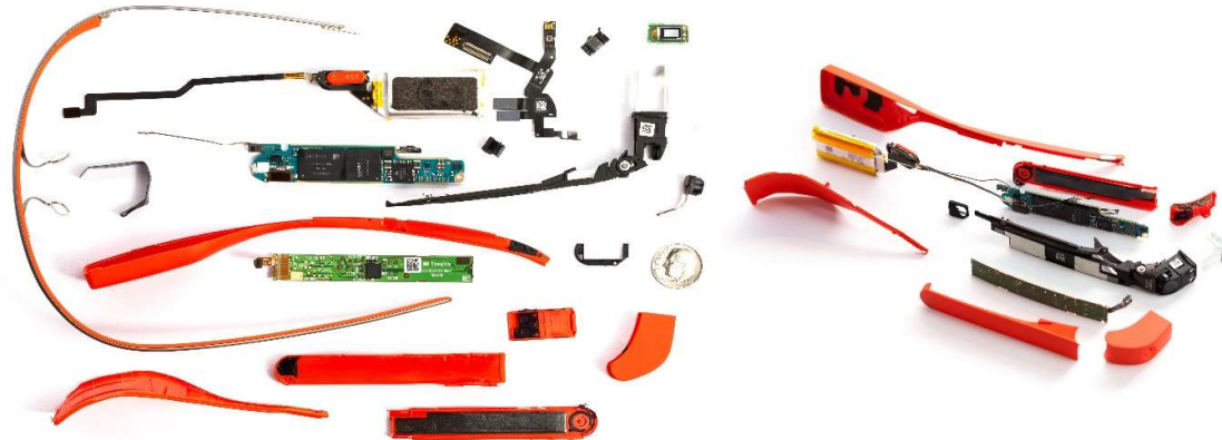
Figure 1(a): All the components of Google Glass. (b) The side opened view of the Google Glass (Google Glass Teardown)
