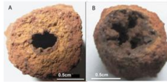
Fig. 3. Cross sections of the tube burrows. A and B are two selected specimens. Color rims around the center hole shows dark inner wall and reddish outer wall with yellow color low oxidized zone in between.
