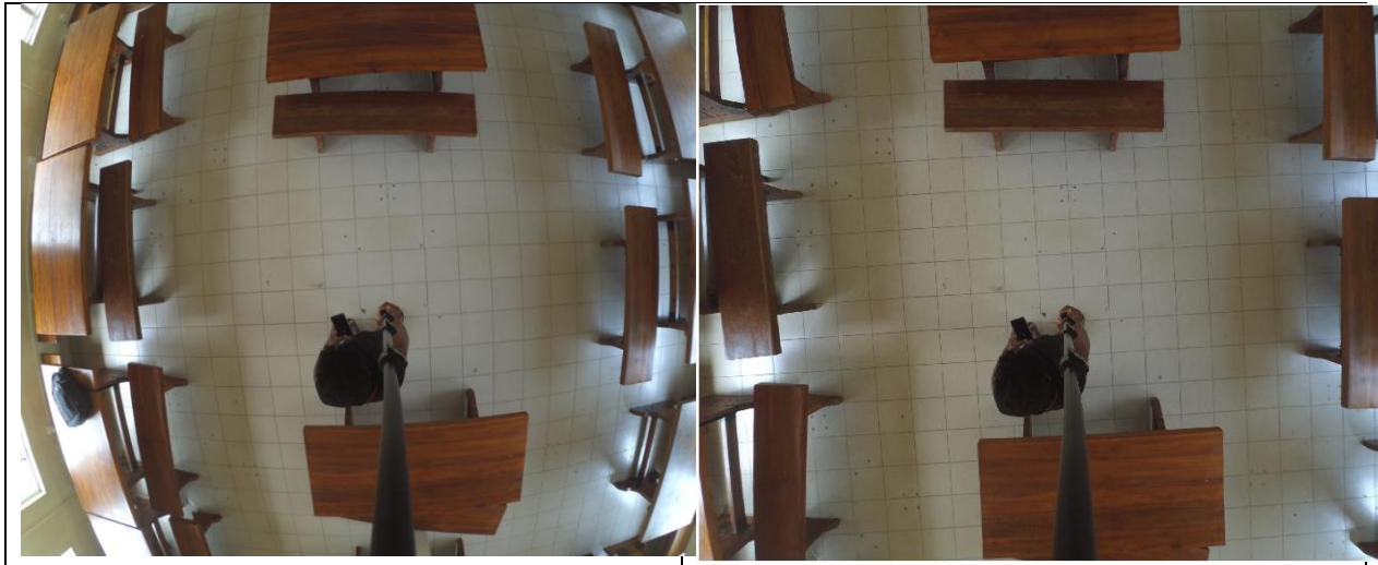
Figure 2: Captured Image of Cafeteria Which Has Distortion in the Edges (Left) and Image of the Cafeteria After Calibration (Right) (This Will Be Used for Further Processing).
