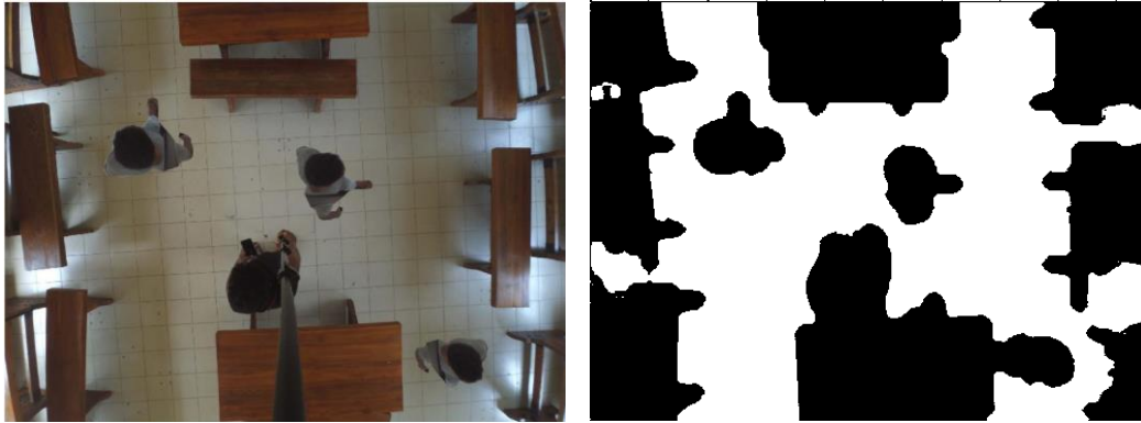
Figure 5: Image with New Objects on The Left and a Binary Image After Detection of All Objects in the Environment.
