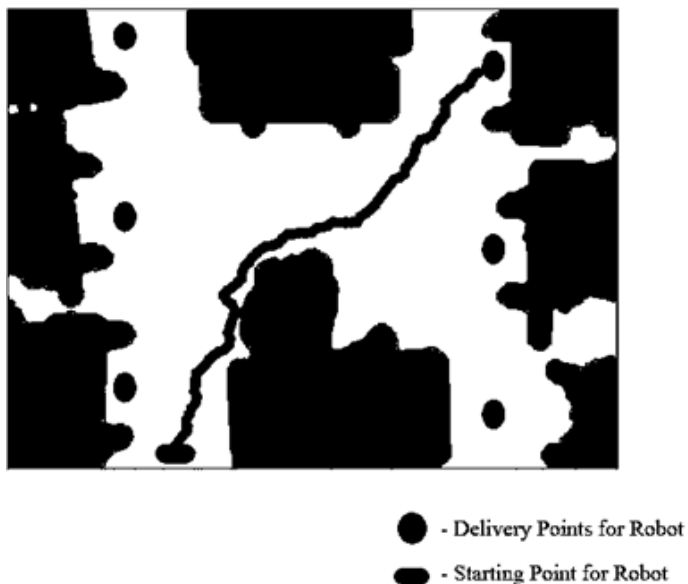
Figure 7: Image Showing the Generated Path from the Robot Starting Point and To One of The Possible Delivery Points
