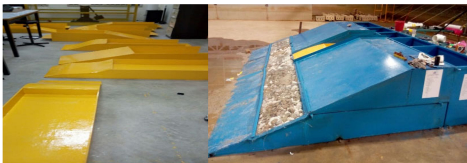
Figure 7. Ramp shapes slot and full assembly model in the basin.
