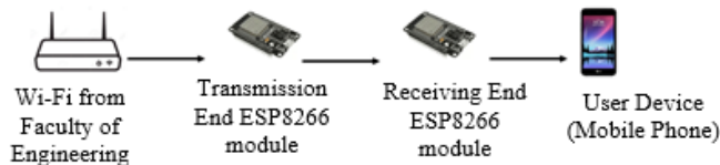
Fig. 13. Experiment 1 Connection Diagram
