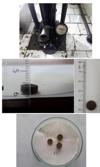
Figure 02: Produced PSP pellets
