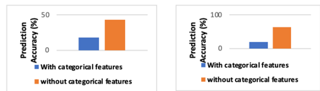
Figure 2: Priority prediction accuracy with and without categorical feature for WSO2 Product-IS (on the left) and Angular (on the right)
