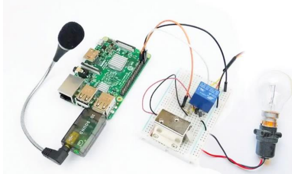
Figure 12. Voice Controlled Room Automation
